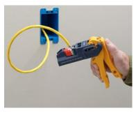
Step 6: Wires will be seated and cut for a solid termination.
