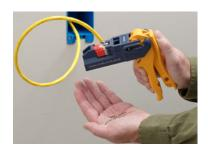
Step 7: Release handle and remove jack from JackRapid tool. Visually verify proper termination.
