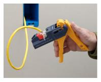
Step 5: Pull trigger completely and remove excess wire prior to releasing trigger.
