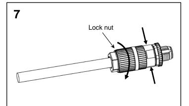
While holding the connecting housing end firmly, twist only the lock nut until fully tightened. Use of 13mm and 17mm open end wrenches may be used to fully seat the o-ring gasket.
