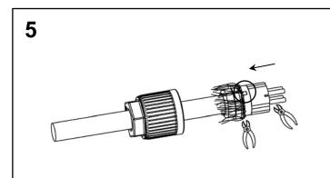
Push splice element onto braid and seal. Trim off excess braid material and cut conductors flush with the splice element.
