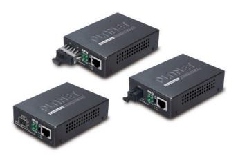
Providing the flexibility of 10/100/1000Mbps Ethernet Media via RJ-45 port and highly stable Gigabit fiber performance, PLANET GT-802, GT-802S, GT-805A and GT-806A/B media converters support conversion between 10/100/1000Base-T and 1000Base-LX/SX network. There are SC/SFP/WDM connectors with single-mode or multi-mode media as required. The Ethernet signal allows three types of segments to connect easily, efficiently and inexpensively.
