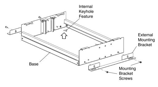
The enclosure base may be mounted to a horizontal or vertical surface using the internal keyhole features or using the external supplied brackets, The external mounting brackets are intended for situations where it is desirable to move the enclosure without needing to remove the cover. The external mounting brackets attach to the sides of the base using the supplied mounting bracket screws.
