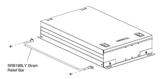
*PANDUIT* strain relief bars (sold separately) may be mounted to the front and rear of the 24 and 48 port enclosures using the threaded holes in the enclosure base and the screws supplied with the strain relief bar.
