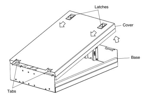
Pull latches simultaneously away from the edge of the cover and lift cover until tabs on opposite side disengage from enclosure base.
