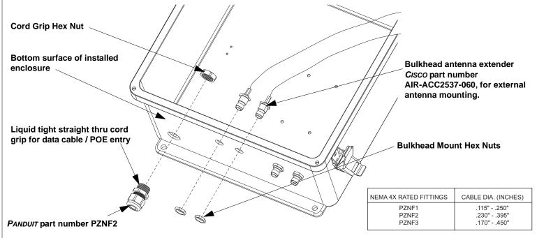
**4.** Install a bulkhead antenna extender, *Cisco* part number **AIR-ACC2537-060** to the bottom surface of the enclosure as shown. Apply RTV silicone to the surface of the collar of the extender to maintain a liquid tight seal. The desired mount hole diameter is 0.53".
