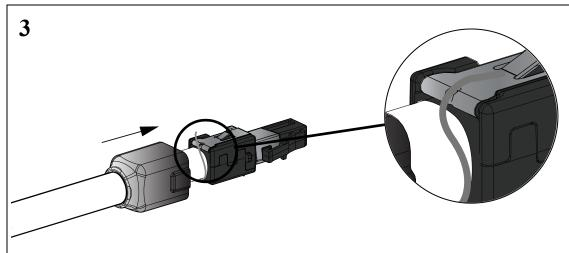
Place drain wire in groove of Shield wrap prior to sliding Outer Cover over wire cap assembly.
