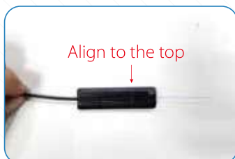
2.6 Put the cable into the cutting clamp
