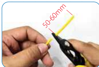
2.2 Strip the cable strengthen layer
