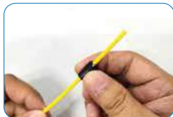
2.1 Put the cable into the boot
