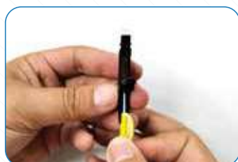
2.9 Put the cable into the boot
