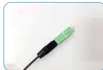
2.12 Lock the fiber (Take off the switch)
