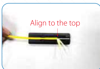
2.6 Put the cable into the cutting clamp
